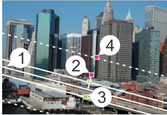
Interactive elements in the Before pane: (1) Center line (for Planar Selection Tool), (2) Rotation handle, (3) Sizing handle, (4) Feathering handle
